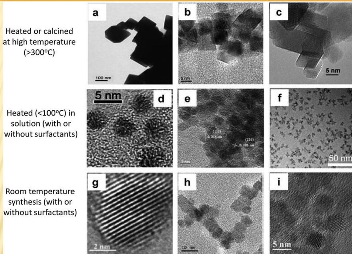
**Figure 3.4** TEM images of CeNPs grouped according to the temperature used during synthesis. Group 1: High temperature (a–c); Group 2: Heated in solvents (d–f); and Group 3: Room temperature (g–i). Reprinted with permission from Ref. [26], Copyright 2012, John Wiley and Sons.
